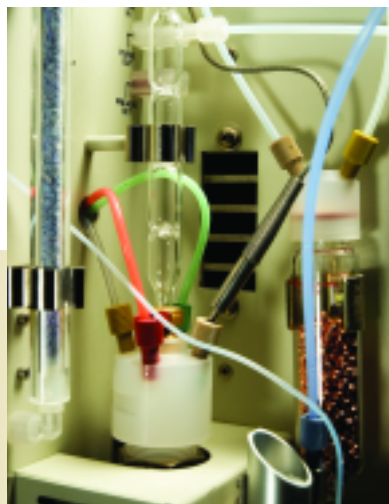
above: Student weighs plant tissue samples for nitrogen isotope analysis. below: This TOC (total organic carbon) analyzer is used to determine carbon isotope ratios in water samples.
